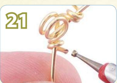
Insert the proper size Wire Rounder Tip into the Battery Operated Bead Reamer for the size of wire used, and press the button to round the sharp edges of the cut piece. Repeat this step on the other cut wire. It is important to round the ends of these wires so there are no sharp edges on the bracelet.
